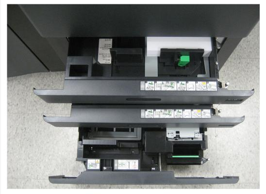
Both length and width guides slide in the drawers when adjusting paper size; plus easy-to-see limit indicators help ensure that paper won't be overloaded in each drawer. (U.S. model pictured)
