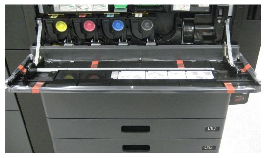
The process for replacing toner is simple and clean; toner can also be changed on the fly. (U.S. model pictured)
