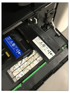
The process for replacing black and erasable blue toner is simple and clean, but toner cannot be replaced on the fly. The device's waste toner container is also user-replaceable.
