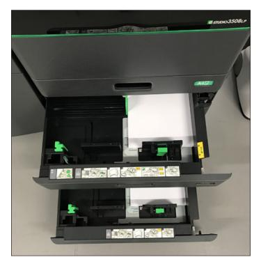
Adjusting the paper drawers for different-sized media is very easy; users simply press the locking clips in and slide to the required size. In addition, paper limit indicators are easy to see which reduces the risk of users overloading the drawers. Administrators can also lock down the size settings for any of the paper drawers so that a user cannot change the size, which helps to prevent errors and misfeeds.
