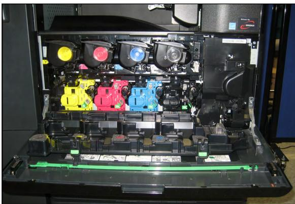
The process for replacing toner is simple and clean, and the device's drums and waste toner are also user-replaceable. (U.S. model pictured)
