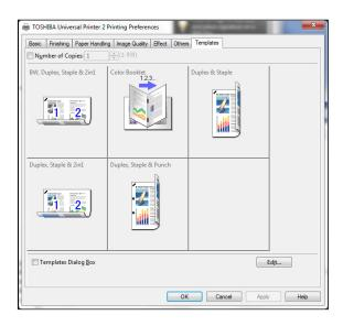
The settings of each template on the Templates tab can be changed and renamed for quick programming of commonly run workflows. (U.S. model pictured)
