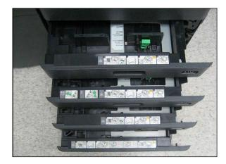
Both length and width guides slide in the drawers when adjusting paper size; plus easy-to-see limit indicators help ensure paper won't be overloaded in each drawer. (U.S. model pictured)
