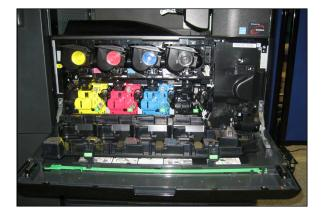
The process for replacing toner is simple and clean, and the device's drums and waste toner are also user-replaceable. (U.S. model pictured)
